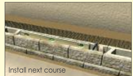
Install AB Reinforcement Grid
