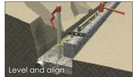
Install facing unit
