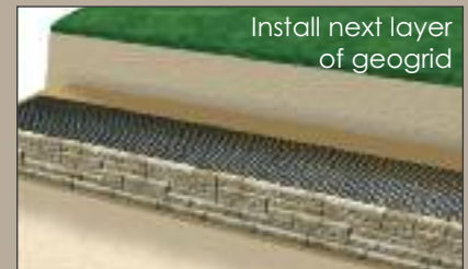
Install next section of pattern
